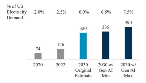
Figure 2: Data Center Electricity Consumption (US, TWhs)<sup>8</sup>
